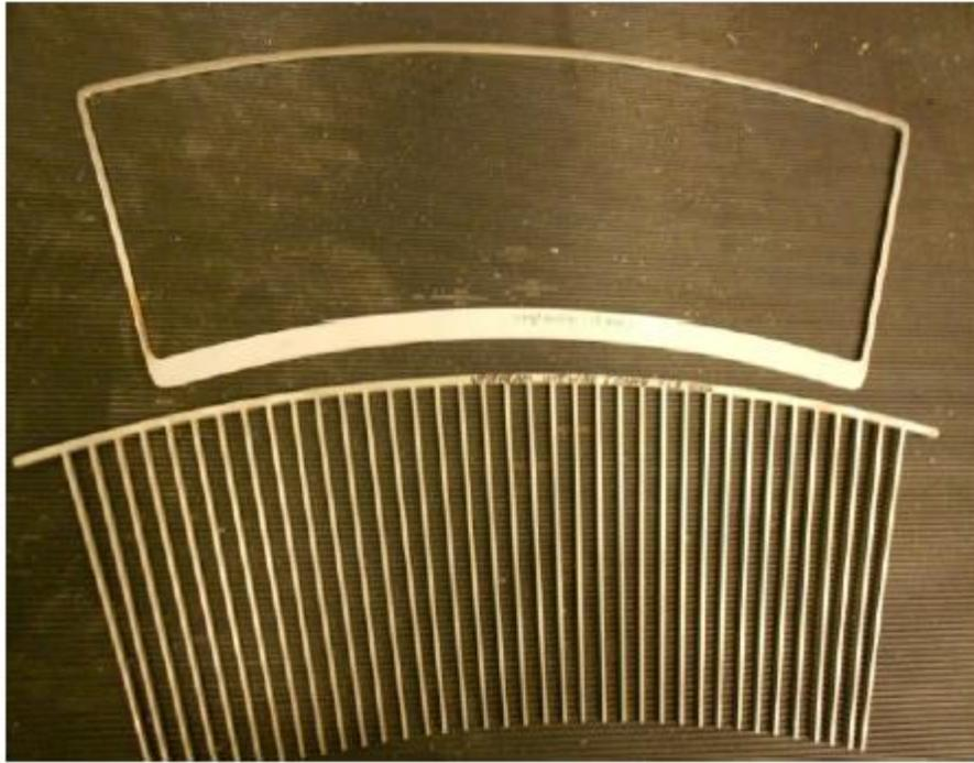
Figure 3-2 Fence (up) and parallel bar (down) turbulence grids (Saha 2012)
